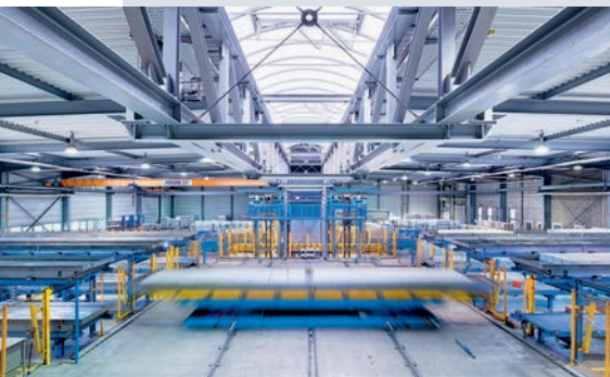
Handling technology for irradiating polymer components on the 10MeV electron accelerator at the Bruchsal site in Germany (© BGS/M. Steur)
