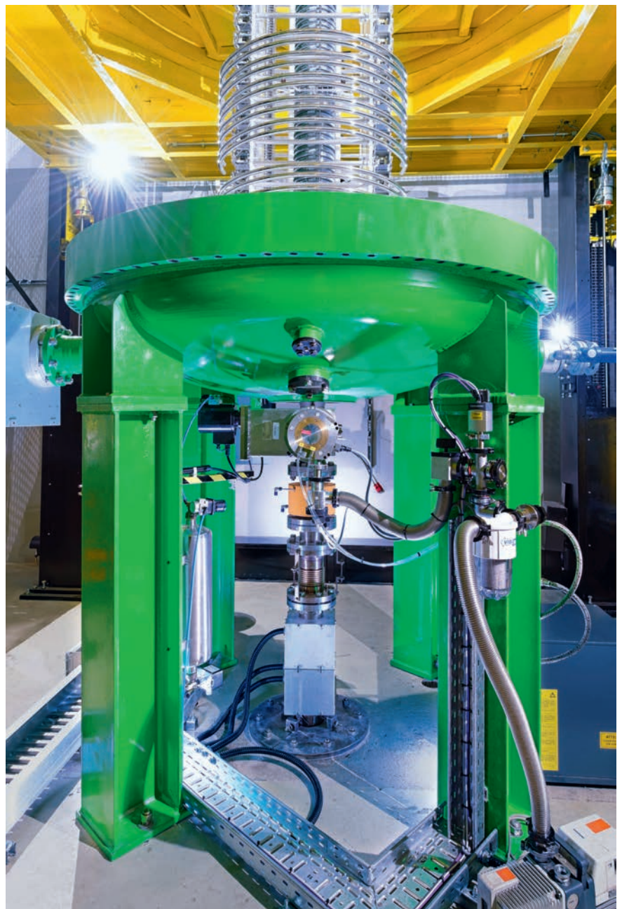
Radiation source: an electron accelerator of 3 MeV maximum energy, operated by BGS Beta-Gamma-Service at its Wiehl site near Cologne, Germany. Electrons released from a hot cathode are collimated into a beam and accelerated via alternating electric fields (© BGS/M. Steur)
